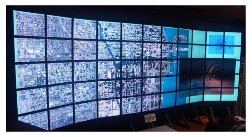
Figure 1. The 100-megapixel LambdaVision tiled-display wall driven by a cluster of 28 computers and run by Scalable Adaptive Graphics Environment (SAGE).
