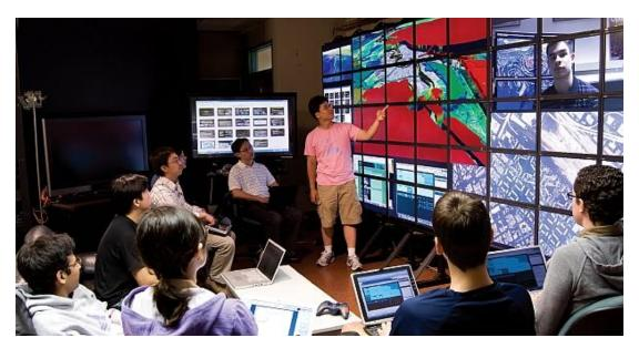
Figure 5. 100-megapixel LambdaVision display used in a research meeting at the Electronic Visualization Laboratory at the University of Illinois at Chicago. The participants stream their desktop screens to the display wall using VNC. Multiple visualizations and HD video of remote participant are streamed to the display wall.
