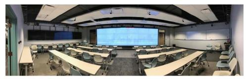
Figure 6. EVL's new Continuum room will combine: a large touch screen wall; a side-wall of 4K displays for extremely high-resolution visual analysis; a passive stereo wall, all driven by SAGE2; and a wall of whiteboards for quick collaborative brainstorming. The room is a quiet space with movable tables and chairs for quick reconfiguration, while a suite of cameras,
