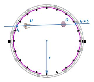
Figure 2 Line  $(\overline{UO})$  between user and sound object, showing wall intercepts  $(I_1, I_2)$  and correct source position  $(S_1)$ .
