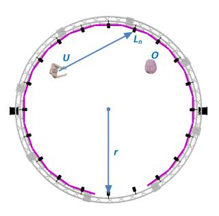
Figure 3 The distance between the user and loudspeaker is divided by the radius of the CAVE2. This ratio is squared to find that loudspeaker's amplitude weighting.
